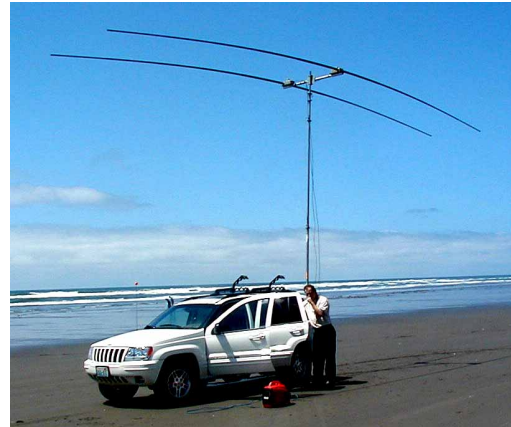
SteppIR yagi shown in portable operation. The antenna took 15 minutes to completely install.
