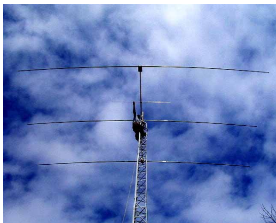
3 element SteppIR yagi shown being utilized in a permanent installation. The SteppIR was a replacement for a log periodic antenna.
