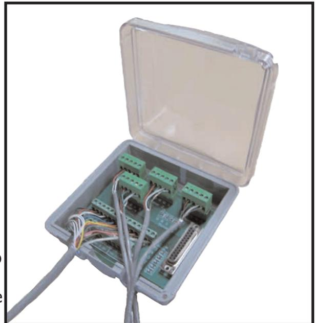
6. Unscrew terminal housing cap, so that you can expose the terminal strip that is inside. Pull out the terminal strip with wires.
